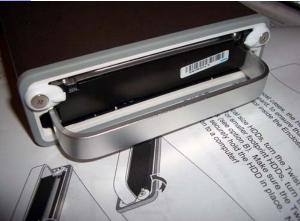
Get a handle on this unusual drive dock! I mean, you affix a brushed aluminum handle to an internal SATA full size 3.5 inch hard drive. This handle is a guide as you insert your drive into a custom powered bay that connects to your Macintosh via FireWire 800/400/USB/eSATA. All necessary cables are provided, colored white.
