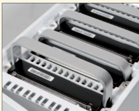
The hard disk drive handles are easy to lift up even when the drive is hot
