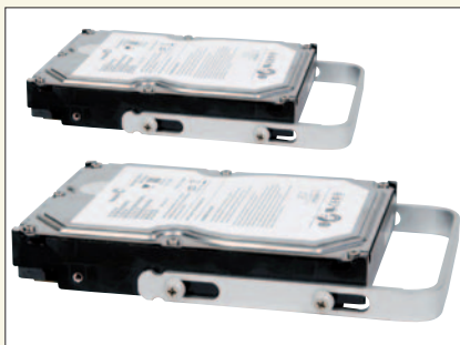
The screw-on guides are easy to install
