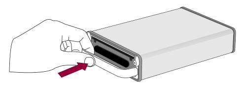
8. For typical-sized hard drive, turn the Twist Locks inward 90 degrees (see option A). For smaller footprint hard drive, turn the Twist Locks inward around 140 degrees (see option B). Make sure the Twist Locks are in the "lock" position and securely hold the hard drive in place. Now, the Enclosure is ready for connection to a computer!
