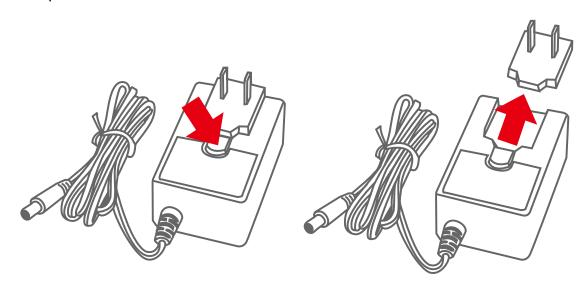
3. Slide the selected Power Plug onto the AC/DC adapter. Now, it is ready to be used!
