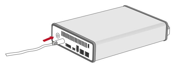
2. Insert the USB 2.0, eSATA, or FireWire 400/800 connector into the corresponding port of the Enclosure, and connect the cable to the host computer.
