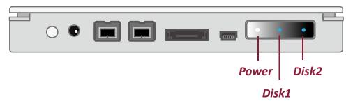
There's no need for any concerns if the Disk LEDs blink or flash in red for a very short period of time during power on. When the HDDs are detected, the Disk LEDs will become and remain in blue.
