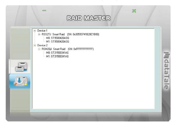
The connected RAID Unit(s) information with Device model of the RAID Unit(s), and serial numbers of each inserted HDDs.
