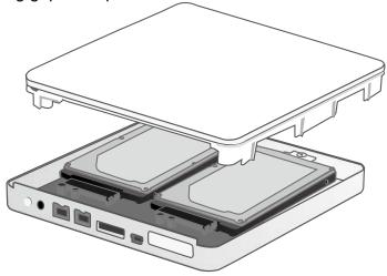
7. Once the Cover is placed on the RAID Unit, use both hands to firmly hold and turn the RAID Unit to its Bottom View. Find the four (4) Casing Screws previously taken out before and re-fasten them in the appropriate screw holes.
