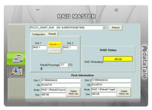
Even if the RAID Unit loses connection to the host, the Rebuild will continue. If the RAID Unit is powered off, the RAID Unit will retain the Rebuild status in its memory. When the RAID Unit is powered "on" again, the Rebuild process will resume from the previous status.
