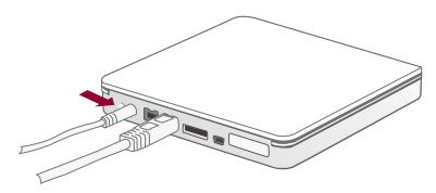
The RAID Unit can also be powered by using only the FireWire 800 cable, without the AC/DC Adapter.
