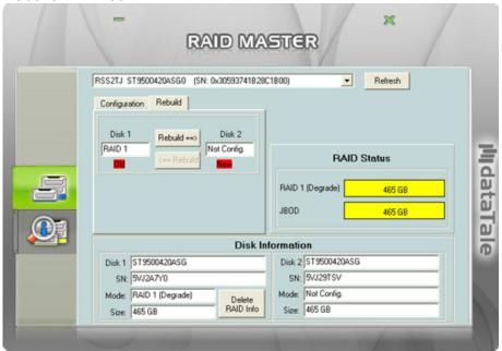
The New HDD may be inserted into either Disk 1 or Disk 2, because the Rebuild feature can be performed in either direction.
