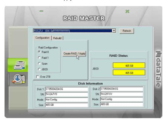
If cannot see what is/are connected as part of the RAID Unit, press the "Refresh" button on top of the first sub-menu (top). The information should appear afterwards.
