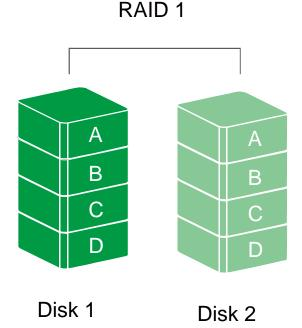
In Mirroring mode, if one of the disks fails, either source or backup, the data is still available. However, if the Old disk fails during the Rebuild process, the data in both disks will be lost.
