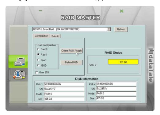
If the host can support more than 2TB HDD(s) storage capacities and the HDD(s) is/are over 2TB, remember to *check* the "Over 2TB" option under the "Configuration" option tab. Please see "Over 2TB" section under Q&As for more information. Please review the "DISK VOLUME OVER 2TB" section of the User's Manual for OS support information
