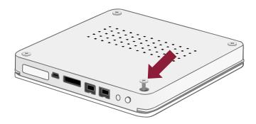
2. Lift the Cover upward to remove it. When opened, the PCBA boards (Printed Circuit Board) should be securely in place inside the RAID Unit.
