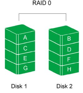
In Striping mode, if one disk in the RAID Unit fails, **all data** in installed disks will be lost.
