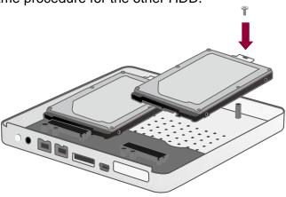
6. Place the RAID Unit facing you. Align the Cover according to the appropriate interface opening gaps and place it on the RAID Unit.
