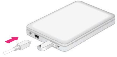
If the LED indicator is red, it is because the host cannot access the HDD and the Secure Key is not inserted. To solve the problem: First, completely unplug the USB cable to power off the Enclosure Kit. Second, insert the Secure Key. Third, re-plug the USB cable to power on the Enclosure again.
