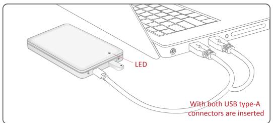
The USB Y-cable provides 2 USB type-A connectors and 1 USB mini-B connector. The 2 USB type-A connectors are inserted into two available USB ports on the computer. The USB Y-cable serves as both power supply and data transfer cable. When the host computer doesn't supply enough power to start up the HDD under only one USB connector, plug in the second type-A connector into the host computer.
