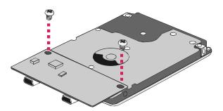
The smaller (Case) screws are for fastening the Enclosure's housing and lid together.
