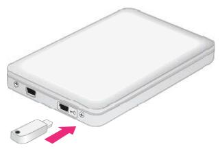
Always plug in the Secure Key **first** every time the Enclosure Kit is connected to a host. The Secure Key may be removed after the host computer detects the Enclosure.
