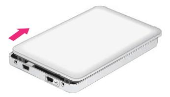
Carefully take out the PCBA board from the Enclosure. Align the SATA connector of the hard drive with the PCBA board. Carefully insert the SATA connector into the slot on the PCBA board until it's firmly connected.
