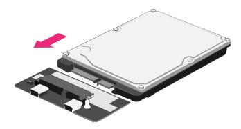
3. Turn the hard drive connected to the PCBA board to its backside. Locate two larger (HDD) screws enclosed inside the package. Tighten the screws in its appropriate holes, ensuring that the hard drive and PCBA alignment is properly maintained.
